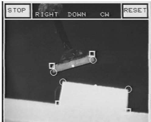
Figure 5. Example of object and environment sensing points (indicated by circles) and the corresponding tracking windows (window centers are represented by squares).
